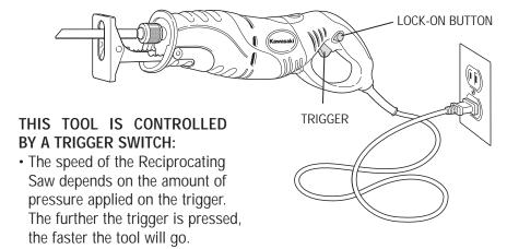
• To maintain a certain speed, pull the "On/Off" trigger to turn the Reciprocating Saw "ON" and engage the lock-on button. To turn the Reciprocating Saw "OFF", release the trigger switch. The lock-on button will automatically reset.
